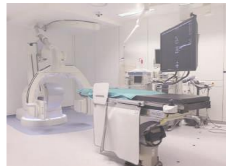
Multi-axis robotic CBCT system ARTIS ZEEGO
